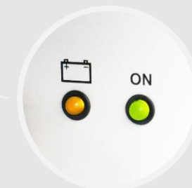
Yellow CHARGE LED indicates battery charging on Control unit
