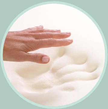
Memory effect of viscoelastic foam
